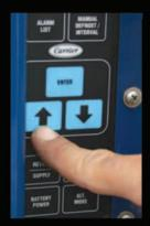
To increase the temperature press and hold the UP arrow
